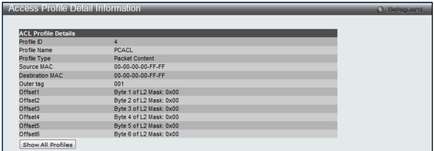
Figure 8-19 Access Profile Detail Information window (Packet Content ACL)
