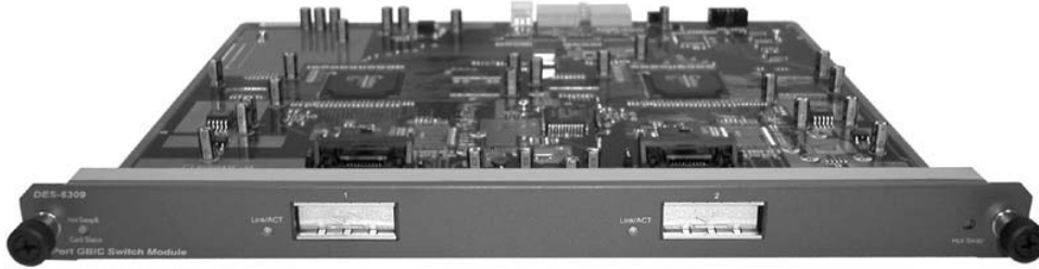
Figure 3- 8. Two-port GBIC Module
