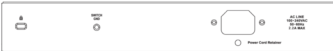
Figure 2-4 – DGS-1100-10MPP Rear Panel
