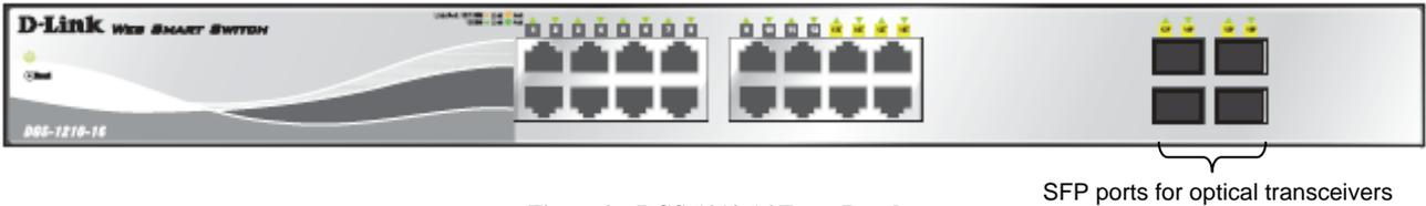
Figure 3 – DGS-1210-16 Front Panel
