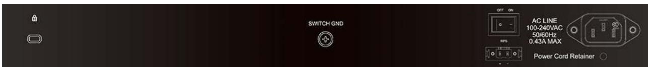
Figure 1.19—DGS-1210-28/ME Rear Panel
