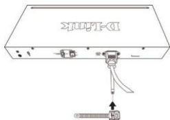
Figure 3-3. Slide the Retainer through the Tie Wrap
