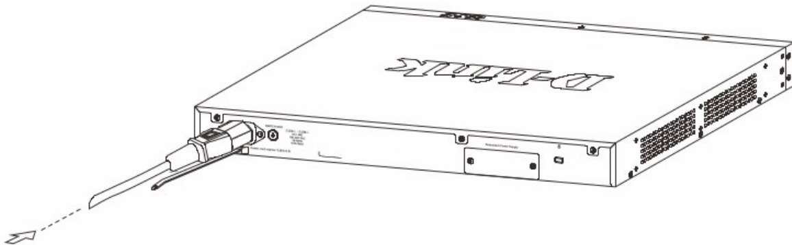
Figure 9 — Connect the power cord to the switch
