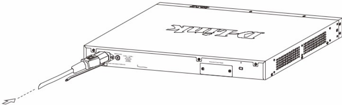
Figure 9 — Connect the power cord to the switch
