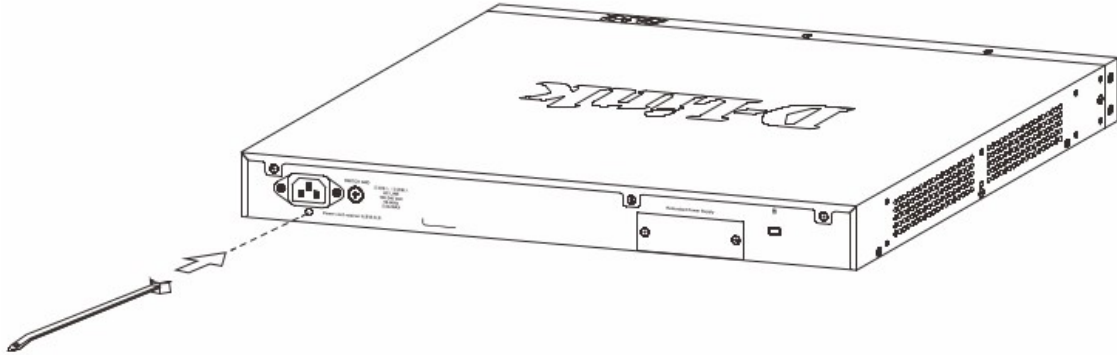
Figure 8 — Insert tie wrap into the switch
