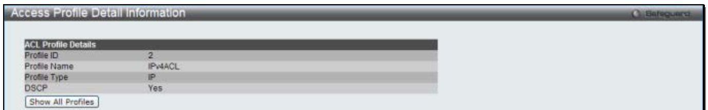
Figure 7-9 Access Profile Detail Information window (IPv4 ACL)
