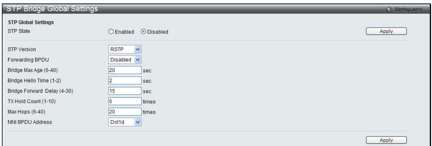
Figure 4-36 STP Bridge Global Settings window
