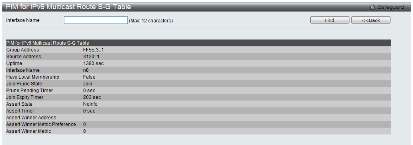
Figure 5-10210 PIM for IPv6 Multicast Route S-G Table- View Detail window
