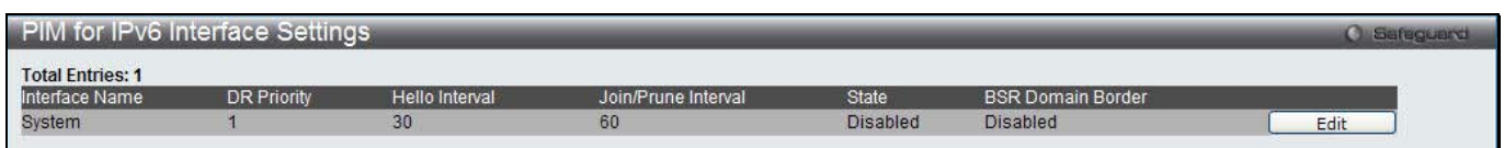
Figure 5-874 PIM for IPv6 Interface Settings window
