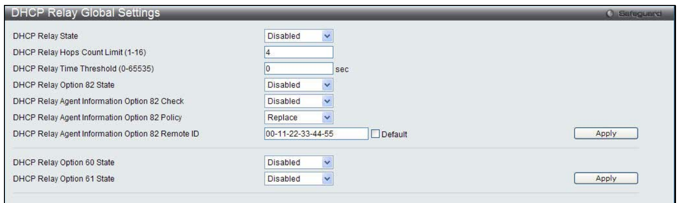
Figure 9-1 DHCP Relay Global Settings window
