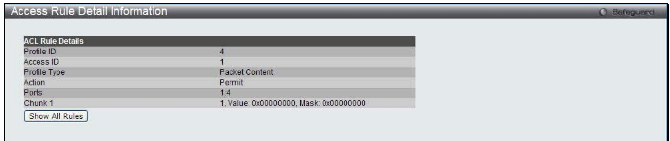
Figure 7-22 Access Rule Detail Information (Packet Content ACL)
