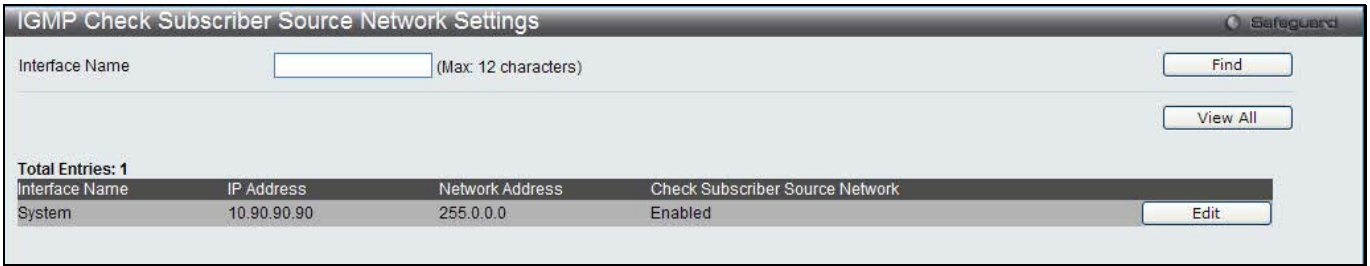
Figure 5-70 IGMP Check Subscriber Source Network Settings window
