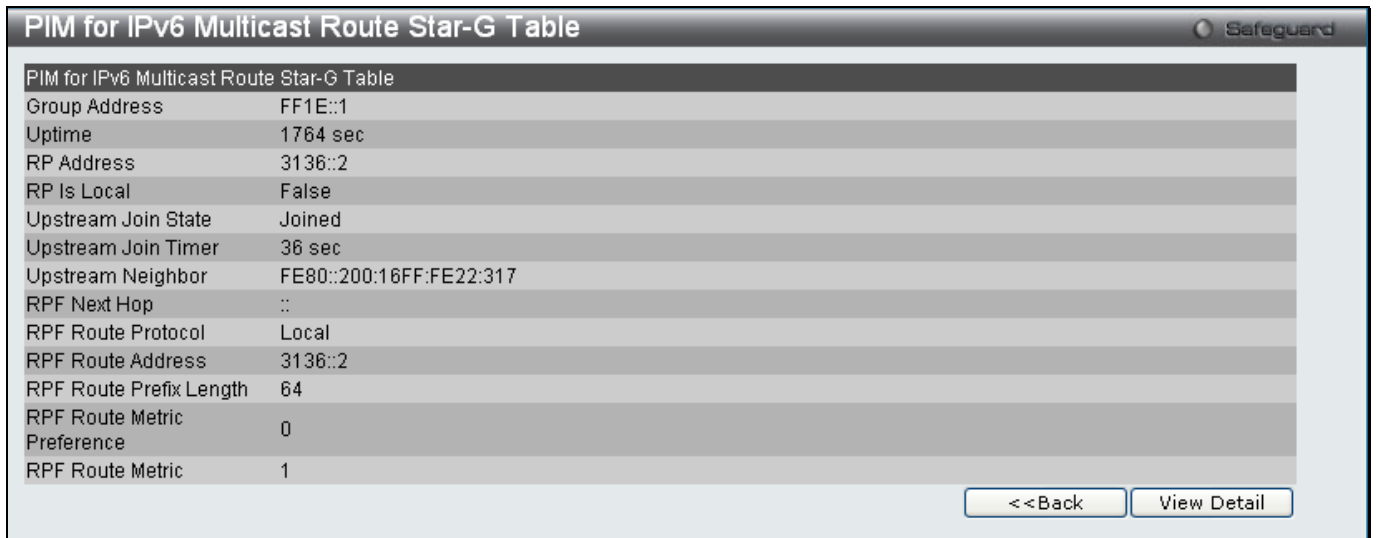
Figure 5-986 PIM for IPv6 Multicast Route Star-G Table - View Detail window
