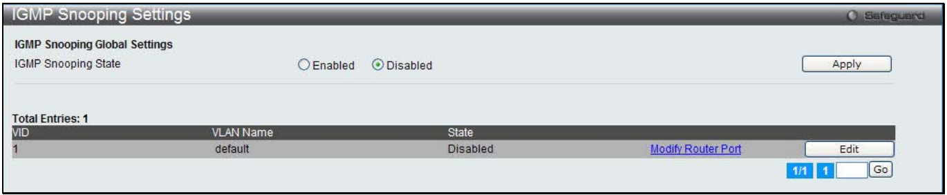
Figure 4-54 IGMP Snooping Settings window
