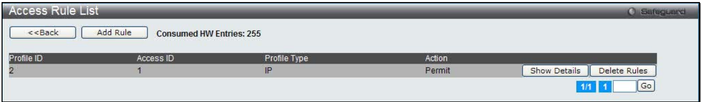
Figure 7-10 Access Rule List window (IPv4 ACL)
