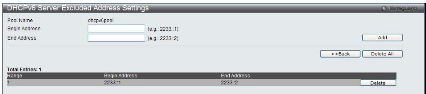
Figure 9-17 DHCPv6 Server Excluded Address Settings window
