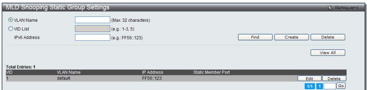
Figure 4-73 MLD Snooping Static Group Settings window
