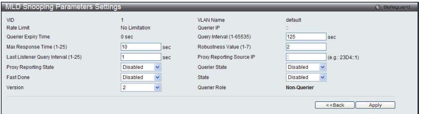
Figure 4-70 MLD Snooping Parameters Settings window
