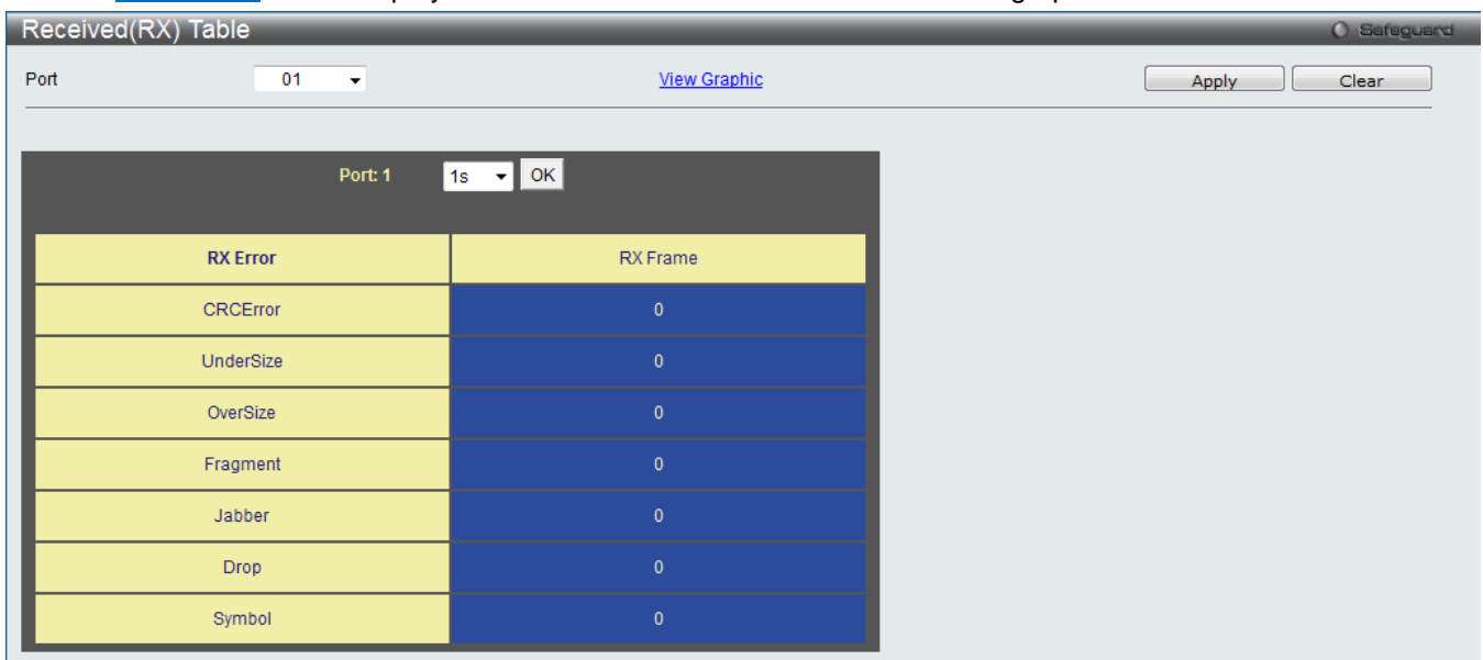
Figure 11-11 RX Error Analysis window (table)
