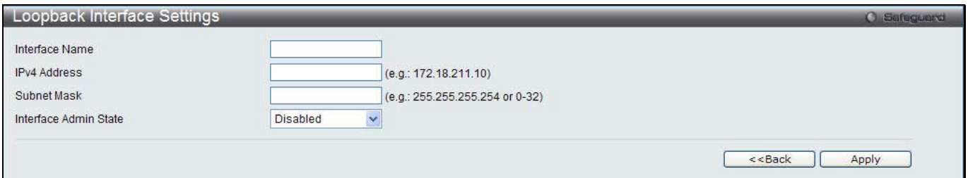
Figure 3-15 Loopback Interface Settings - Add/Edit window
