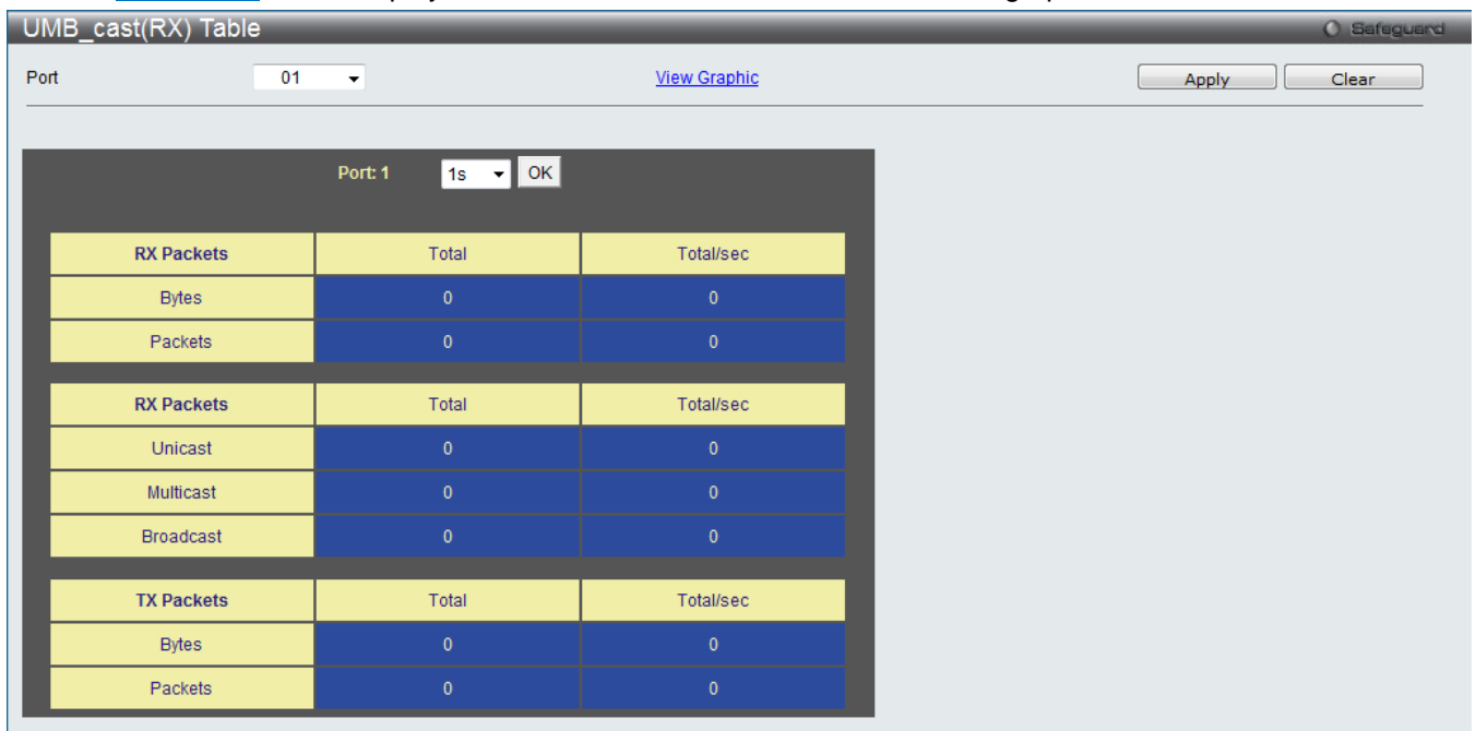
Figure 11-7 RX Packets Analysis window (table for Unicast, Multicast, and Broadcast Packets)
