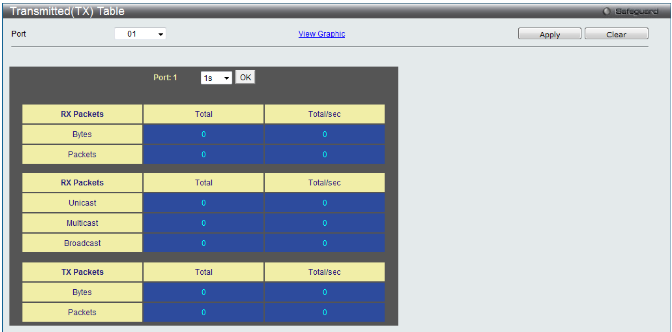
Figure 11-9 TX Packets Analysis window (table for Bytes and Packets)
