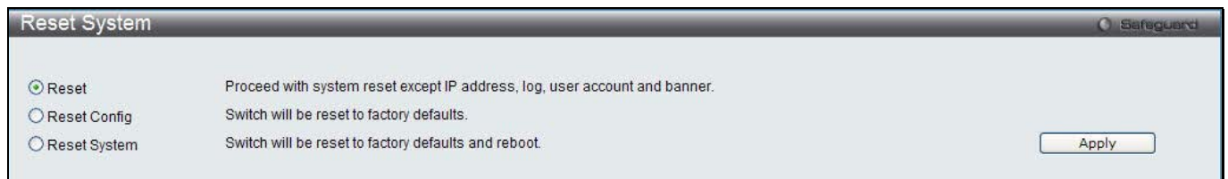
Figure 12-19 Reset System window
