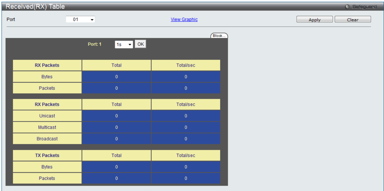
Figure 11-5 RX Packets Analysis Table window
