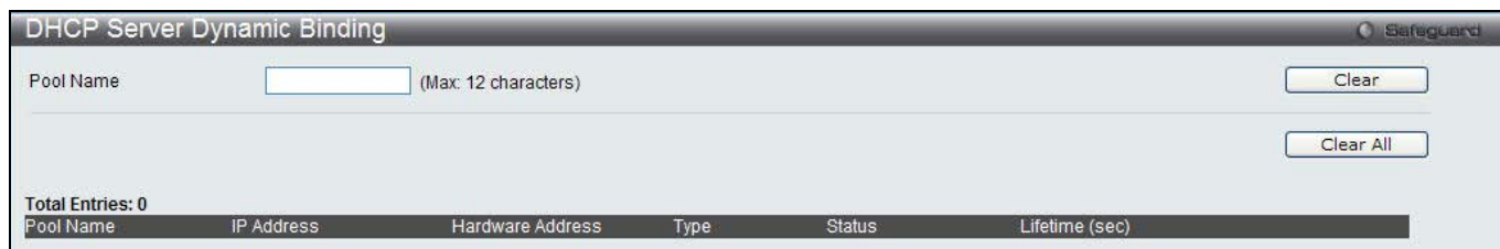
Figure 9-13 DHCP Server Dynamic Binding Window
