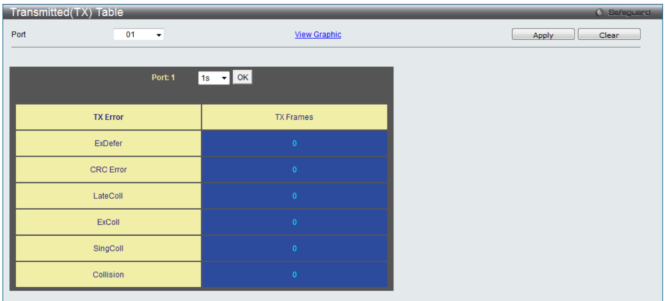
Figure 11-13 TX Error Analysis window (table)
