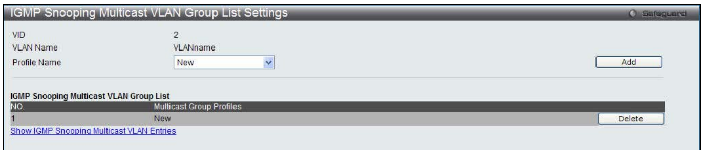
Figure 4-84 IGMP Snooping Multicast VLAN Group List Settings window
