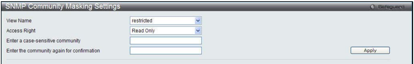
Figure 3-48 SNMP community Masking Settings window
