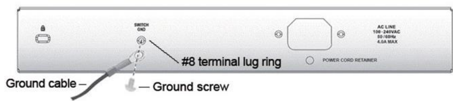
Figure 2.10 – Connect a Grounding Cable
