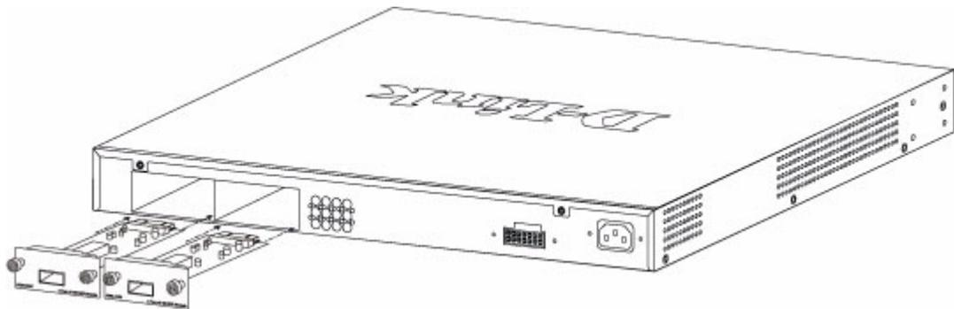
Now tighten the two screws at adjacent ends of the module into the available screw holes on the Switch. The upgraded Switch is now ready for use.
