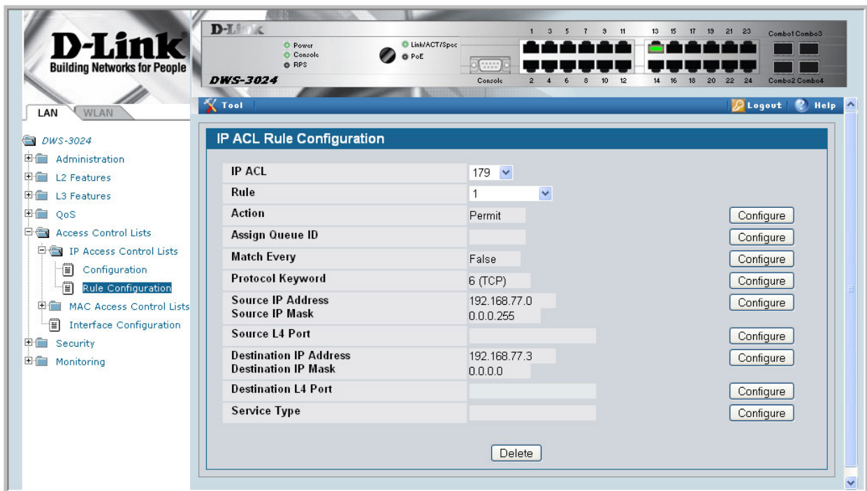
Figure 51. IP ACL Rule Configuration Page - Rule with Protocol and Source IP Configuration
