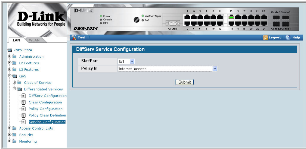
Figure 94. DiffServ Service Configuration
