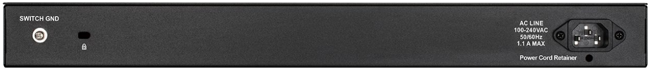
Figure 1.8 – DXS-1210-16TC Rear Panel
