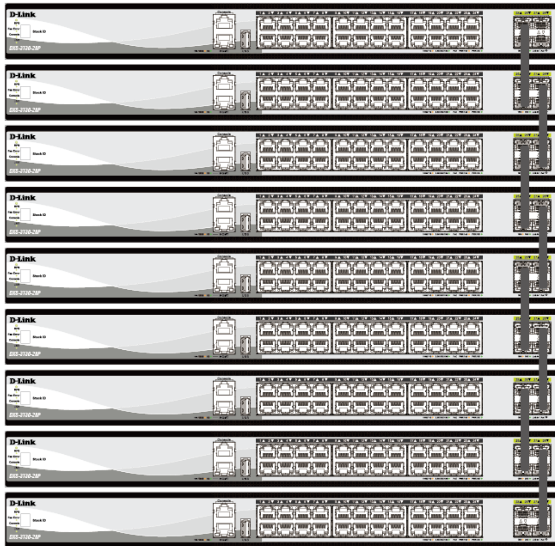
Figure 0-3 Duplex Chain stacking topology (SFP28 ports)
