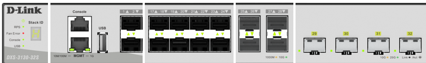
Figure 2-6 LED indicators for the DXS-3130-32S
