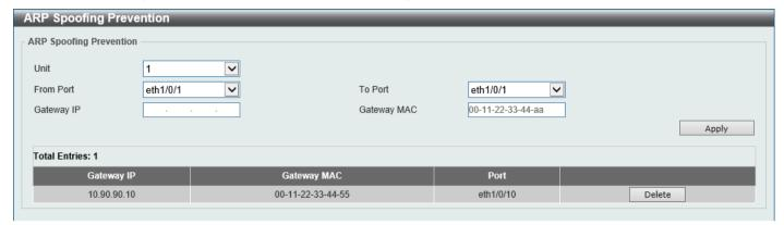
Figure 9-68 ARP Spoofing Prevention Window
