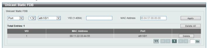
Figure 5-1 Unicast Static FDB Window
