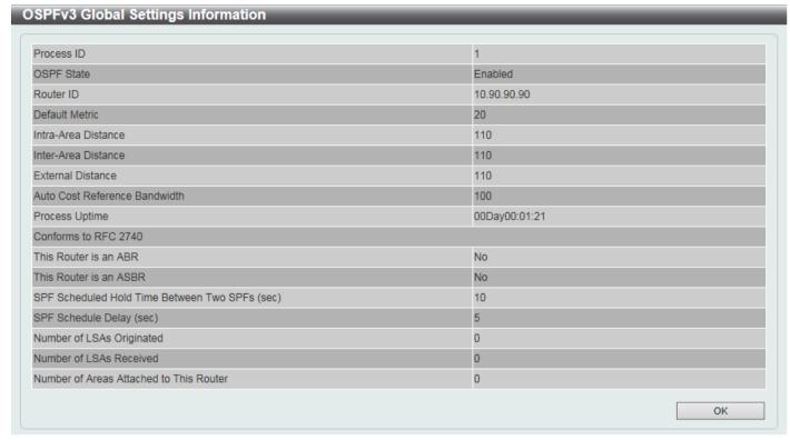
Figure 6-54 OSPFv3 Process Settings (Process ID) Window
