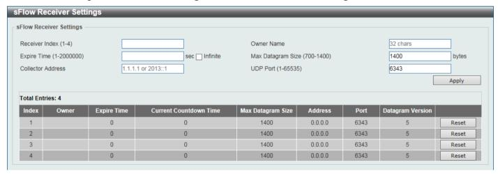
Figure 11-19 sFlow Receiver Settings Window
