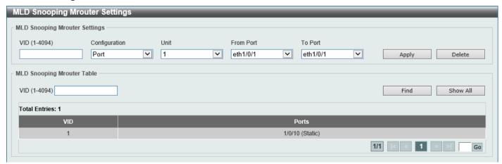
Figure 5-94 MLD Snooping Mrouter Settings Window
