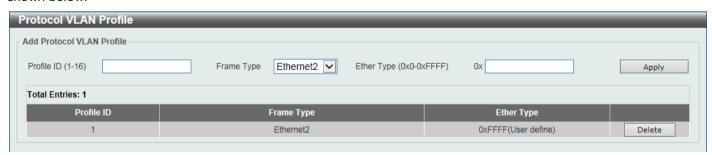
Figure 5-19 Protocol VLAN Profile Window
