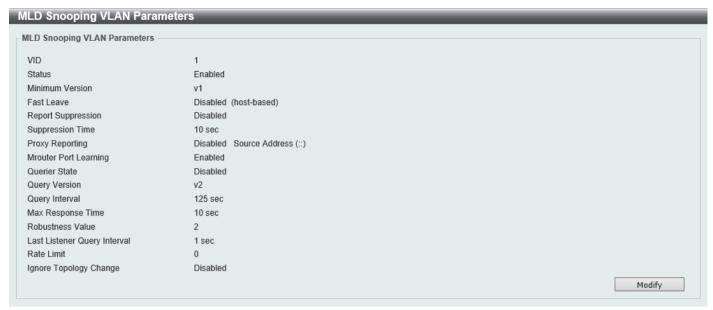
Figure 5-88 MLD Snooping Settings (Show Detail) Window
