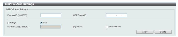
Figure 6-57 OSPFv3 Area Settings (Stub) Window
