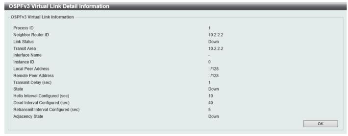
Figure 6-64 OSPFv3 Virtual Link Settings (Process ID) Window
