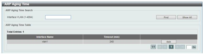
Figure 6-1 ARP Aging Time Window
