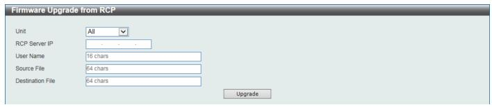
Figure 13-5 Firmware Upgrade from RCP Window
