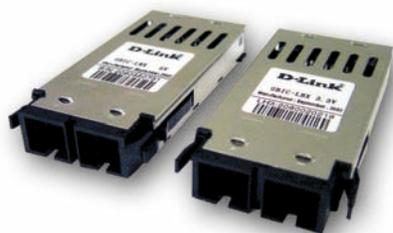
D-Link's new line of Gigabit Interface Converters (GBICs) and Small Form-Factor Pluggables (SFPs) transceivers represent an industry leading combination of performance and affordability. D-Link's new Gigabit transceivers are available in two form-factors: standard (GBIC) or (SFP)/mini-GBIC.
