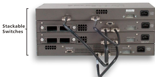
xStack™ - Ring (Bus) Architecture
