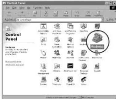
**Step 6** Check "Don't detect my modem....." item and click **Next >** to install a new modem.
