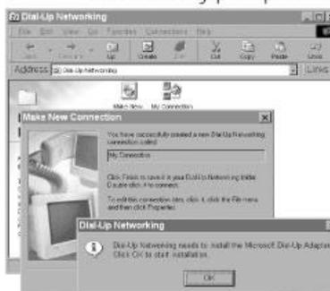
**Step 11** After the 33600 bps modem is installed, open the Dial-Up Networking folder in Windows to build a new connection.
