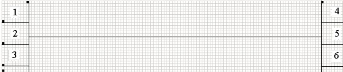
LCD will leave 20 columns for displaying icons, 10 columns on each side. Each icon size is 10x8 . So there're six positions, numbered from No.1 to No.6, on LCD for indication of different status.
