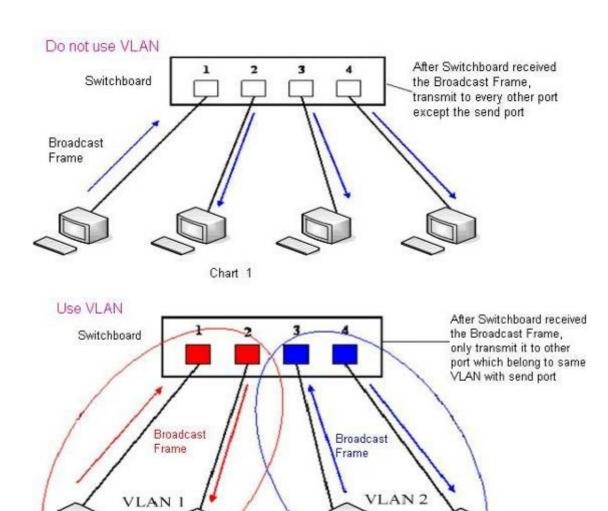
In chart 1, there is a layer 2 switch without setting VLAN. Any broadcast frame will be transmitted to the other ports except the send port. For example, a broadcast information is sent out from port 1 then transmitted to port 2,3and 4.
