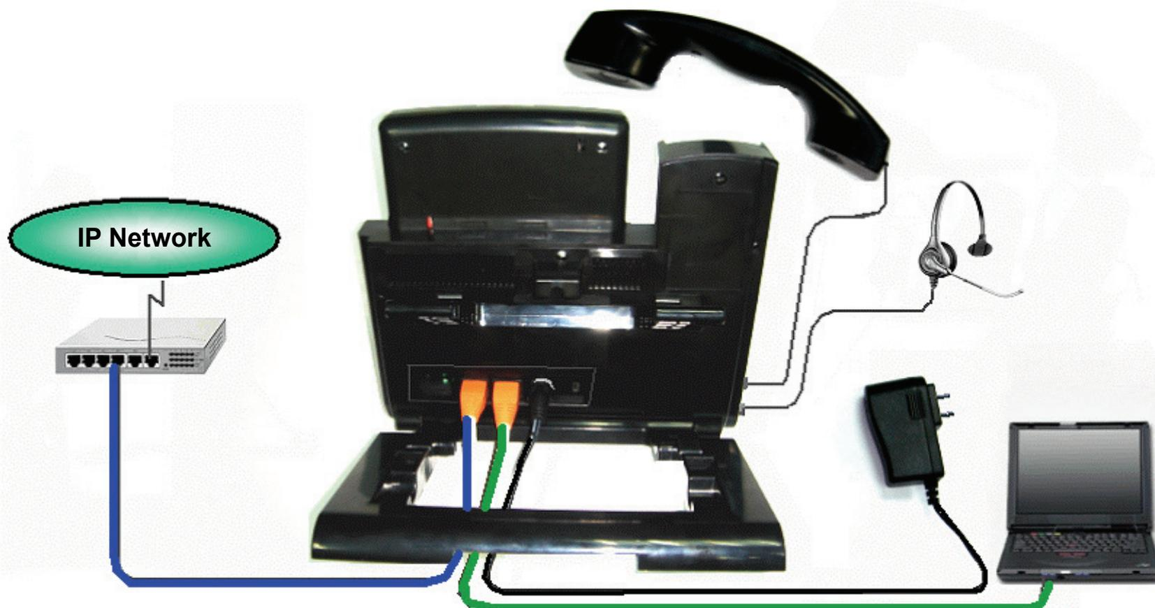
4. Connect an Ethernet cable to the LAN port on the phone and connect the other end to an Ethernet Switch port that is linked to an IP network (see figure above).
