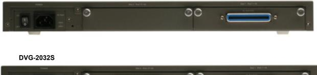
**FXS Connector:** Connect to your phones using attached phone cabling. **Ground:** A conducting connection with the earth. Connect with the ground so as to make the earth a part of an electrical circuit using metal wire. **Power Receptor:** Receptor for AC power 100V- 240V.
