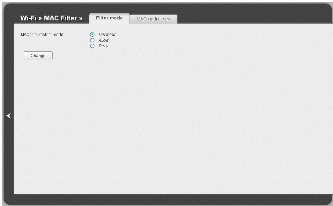
Figure 46. The MAC filter for the wireless network.
