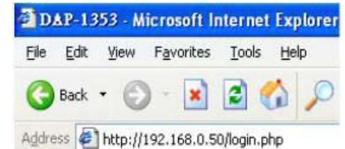
**Note:** If you have changed the default IP address assigned to the DAP-1353, make sure to enter the correct IP address.
