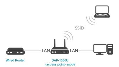
The DAP-1360U device in the "access point" mode is connected to the wired router. Computers connect to DAP-1360U via wireless or wired connection.
