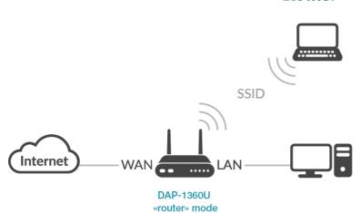
The DAP-1360U device in the "router" mode is connected to a private Ethernet line or to a cable or DSL modem. Computers connect to DAP-1360U via wireless or wired connection. It is necessary to specify the same encryption parameters and the channel of the wireless network for DAP-1360U and computers with Wi-Fi adapters. In addition, it is necessary to configure a WAN connection for DAP-1360U.
