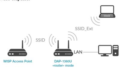
The DAP-1360U device in the "router" mode is connected to a WISP access point via wireless connection. Computers connect to DAP-1360U via wireless or wired connection.
