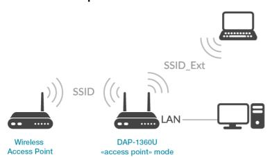
The DAP-1360U device in the "access point" mode is connected to an access point via wireless connection. Computers connect to DAP-1360U via wireless or wired connection. It is necessary to configure the same parameters of the wireless connection (the name of the wireless network, encryption parameters, and the channel) for DAP-1360U and the remote access point.
