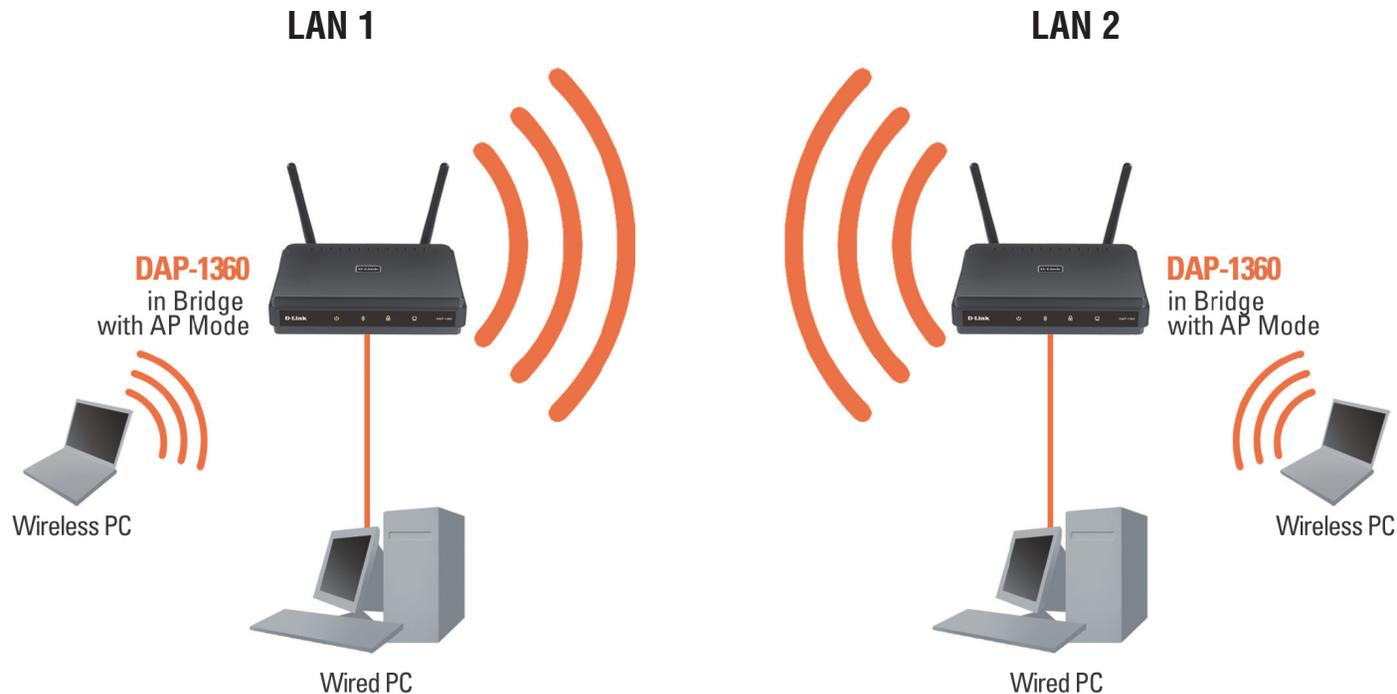
**Connecting Two Separate LANs Together Through Two DAP-1360 Units
