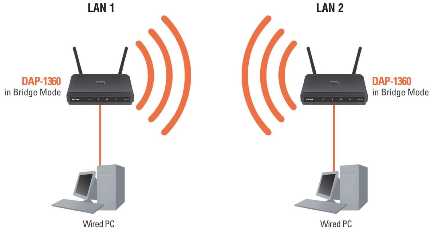
**Connecting Two Separate LANs Together Through Two DAP-1360 Units
