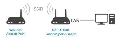
The DAP-1360U device in the "access point" mode is connected to an access point via wireless connection. Computers connect to DAP-1360U via wireless or wired connection. It is necessary to configure the same channel of the wireless connection for DAP-1360U and the remote access point. Other parameters of the wireless network of DAP-1360U do not depend upon the settings of the remote access point.
