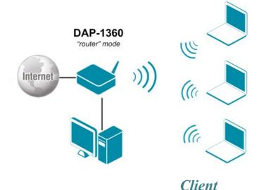
The DAP-1360 device in the "router" mode is connected to a private Ethernet line or to a cable or DSL modem. Computers connect to DAP-1360 via wireless or wired connection. It is necessary to specify the same encryption parameters and the channel of the wireless network for DAP-1360 and computers with Wi-Fi adapters. In addition, it is necessary to configure a WAN connection for DAP-1360.
