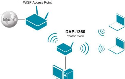
The DAP-1360 device in the "router" mode is connected to a WISP access point via wireless connection. Computers connect to DAP-1360 via wireless or wired connection. It is necessary to configure the same channel of the wireless connection for DAP-1360 and the WISP access point. Other parameters of the wireless network of DAP-1360 do not depend upon the settings of the WISP access point. In addition, it is necessary to configure a WAN connection for DAP-1360.
