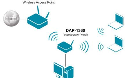
The DAP-1360 device in the "access point" mode is connected to an access point via wireless connection.
