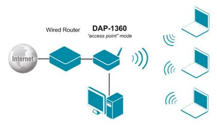
The DAP-1360 device in the "access point" mode is connected to the wired router. Computers connect to DAP-1360 via wireless or wired connection. It is necessary to specify the same encryption parameters and the channel of the wireless network for DAP-1360 and computers with Wi-Fi adapters.
