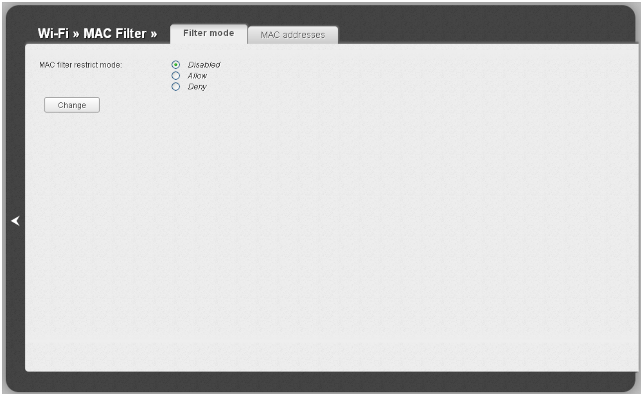
Figure 126. MAC filters for the wireless network.
