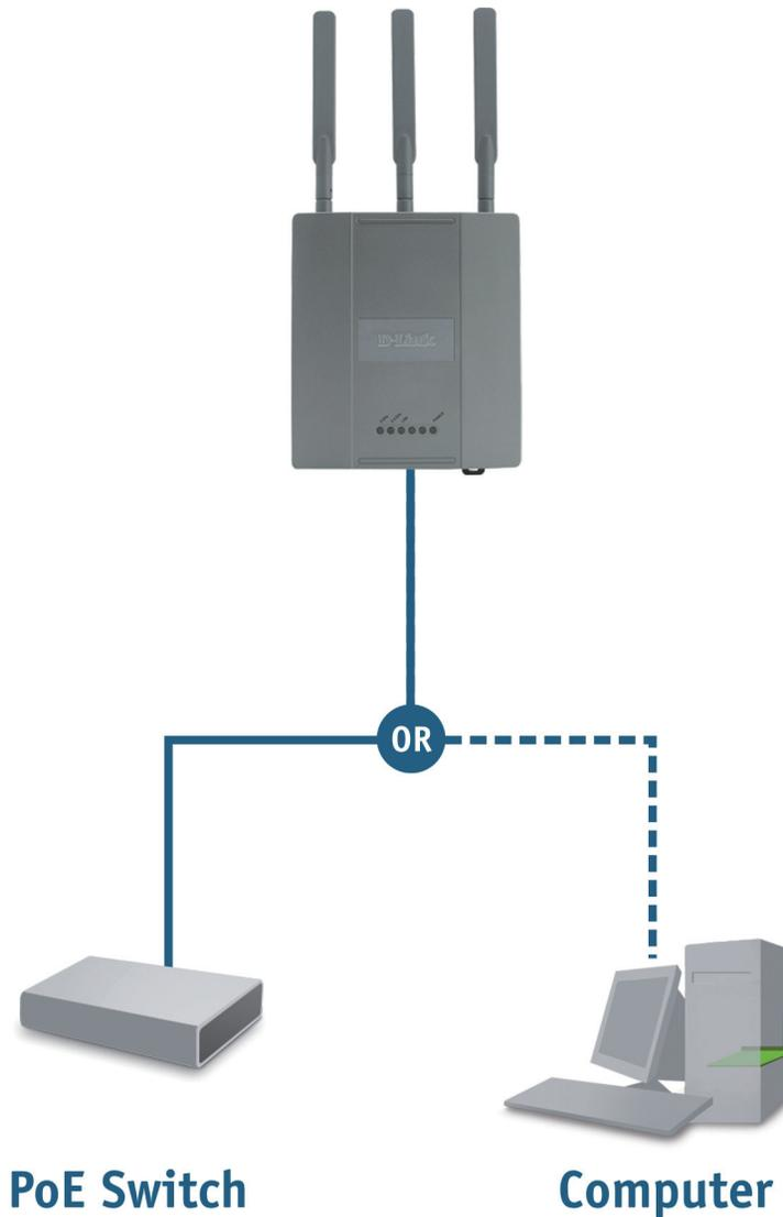
Connect one end of an Ethernet cable (included with your package) to the LAN port on the DAP-2590 and the other end of the Ethernet cable to either your computer or to your PoE switch. The AP can be powered on by a PoE switch or by the power adapter shipped with the AP.
