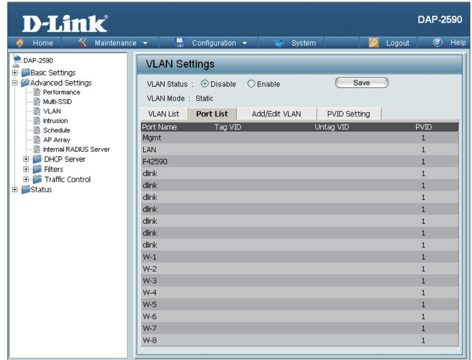
The screenshot shows the D-Link DAP-2590 web interface. The 'VLAN Settings' page is active, with the 'Port List' tab selected. The interface includes a navigation menu on the left and a main content area. The 'VLAN Settings' section shows 'VLAN Status' set to 'Disable' and 'VLAN Mode' set to 'Static'. Below this, there are tabs for 'VLAN List', 'Port List', 'Add/Edit VLAN', and 'PVID Setting'. The 'Port List' tab displays a table with the following data:
