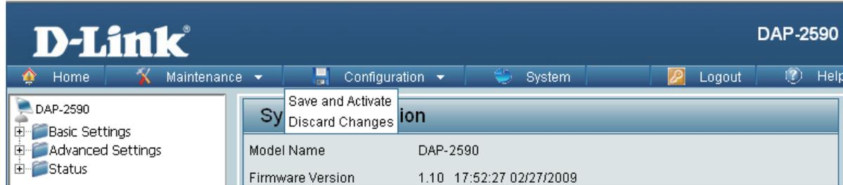
The drop-down Configuration menu allows users to save the current changes and reboot the DAP-2590 by clicking "Save and Activate".
