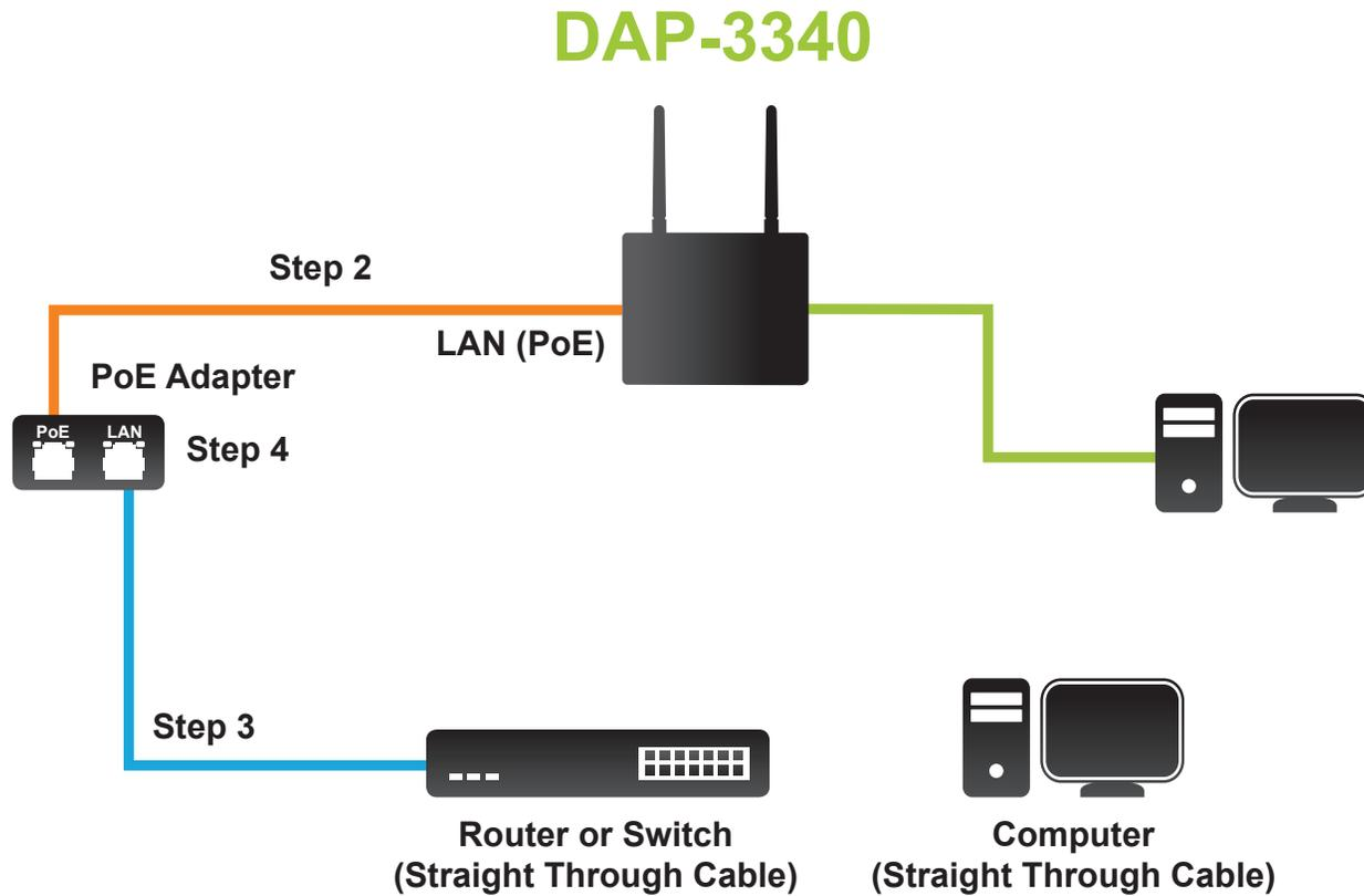
Connect one end of an Ethernet cable (included with your access point) to the LAN port on the DAP-3340 and the other end of the Ethernet cable to PoE power adapter.
