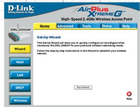
The Web-based configuration interface of the DWL-2000AP allows you to reconfigure the AP in any one of its four operating modes (see left); as well as to apply other management settings.
