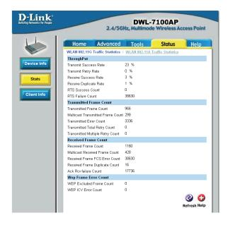
**WLAN 802.11a** This window displays the statistics of the **Traffic Statistics:** IEEE802.11a network.
