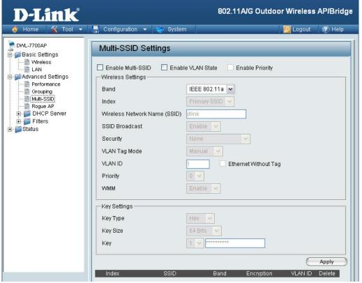
If you want to configure the Guest and Internal networks on Virtual LAN (VLAN), the switch and DHCP server you are using must also support VLANs. As a prerequisite step, configure a port on the switch for handling VLAN tagged packets as described in the IEEE802.1Q standard.
