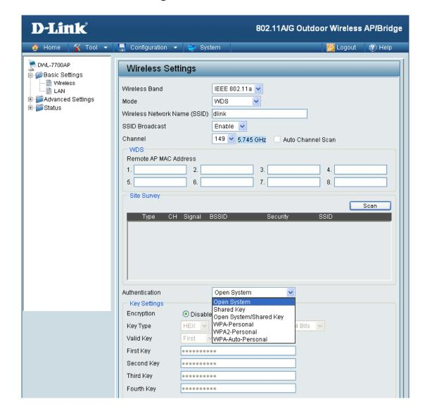
In WDS, the DWL-7700AP wirelessly connects multiple networks, without functioning as a wireless AP.
