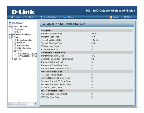
WLAN 802.11a | This page displays statistics for data throughput, transmitted and received **Traffic Statistics:** frames, and WEP frame errors for the 802.11a wireless network.
