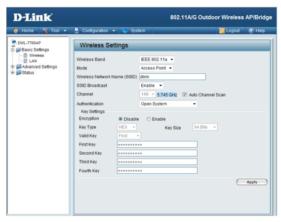
**Encryption:** Select **Enabled** to enable WEP encryption.
