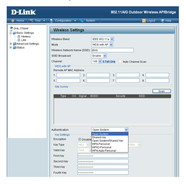
In WDS with AP mode, the **DWL-7700AP** wirelessly connects multiple networks, while still functioning as a wireless AP. WDS (Wireless Distribution System) allows access points to communicate with one another wirelessly in a standardized way. It can also simplify the network infrastructure by reducing the amount of cabling required. Basically the access points will act as a client and an access point at the same time.
