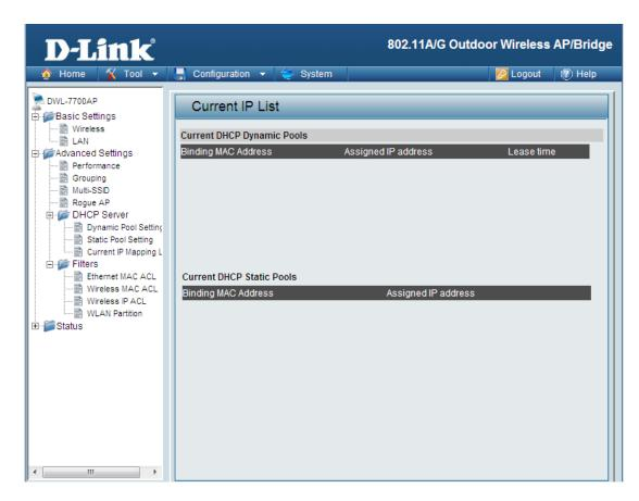
This screen displays information about the current DHCP dynamic and static IP address pools. This information is available when you enable the DHCP function of the **DWL-7700AP** and assign dynamic and static IP address pools.
