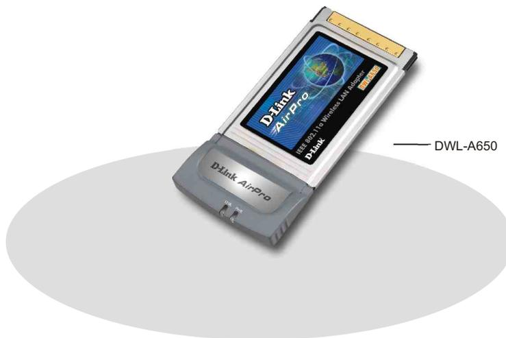
Up to 54Mbps standard transmission speed, 72Mbps Turbo mode, wireless LAN for notebook PC.
