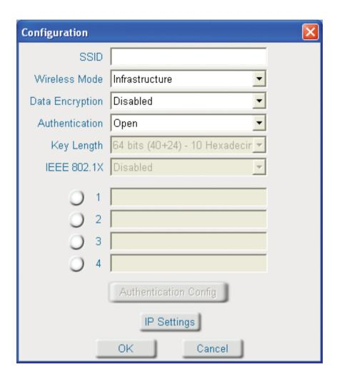
In this window you can configure all the properties of a profile in order to connect with a network of your choice.
