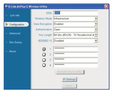
**SSID:** The Service Set Identifier is the name assigned to the wireless network. The factory SSID setting is set to **default**. Make changes here to match the SSID on existing Wireless Router or Access Point.
