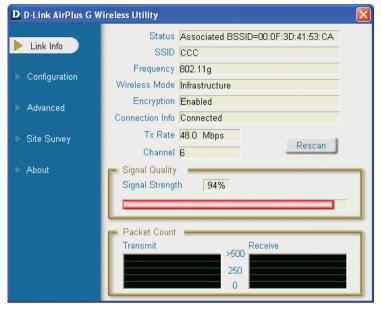
**Status:** Displays the MAC Address of the Access Point that is associated with the DWL-G510.
