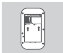
3. Insert the SIM card into the SIM card slot as shown, ensuring the gold contacts are facing down.
