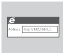
2. Use a web browser to go to **192.168.0.1** to log in to the router's configuration interface. The default username is **admin**, and the password should be left blank.
