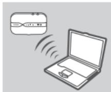
1. Use your PC's wireless adapter to connect to the **dlink\_DWR-932C\_xxxx** wireless network. The wireless network name (SSID) and password are printed on the label under the battery.
