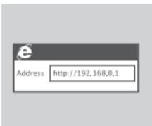
2. Use a Web Browser to **192.168.0.1** to log in to DWR-932C's configuration interface. The default username is **admin**, and the password should be left blank.
