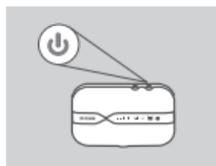
6. Press and hold the power button for four seconds to turn on the device. Once the power LED icon lights up solid green you may proceed with configuration.
