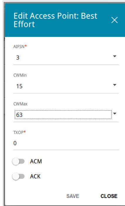
Figure 46. The window for changing parameters of the WMM function.
