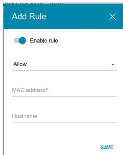
Figure 57. The window for adding a rule for the MAC filter.
