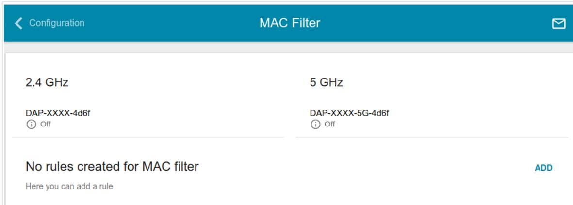
Figure 49. The page for configuring the MAC filter for the wireless network.
