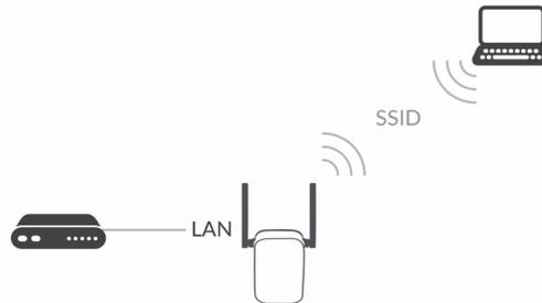
Figure 21. Selecting an operation mode. The **Access point** mode.
