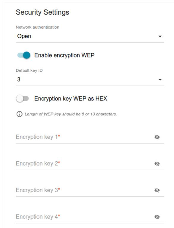
Figure 40. The **Open** value is selected from the **Network authentication** drop-down list.
