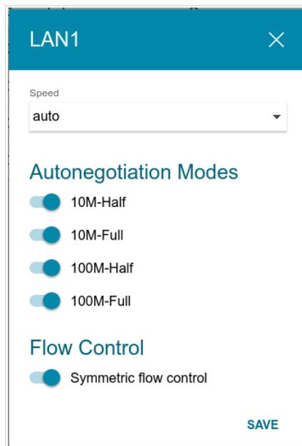
Figure 55. The window for changing the settings of the extender's port.
