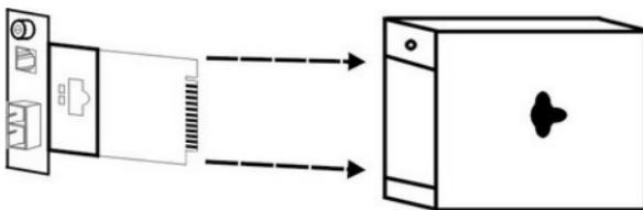
First, install the converter onto a carrier supplied with the chassis:
