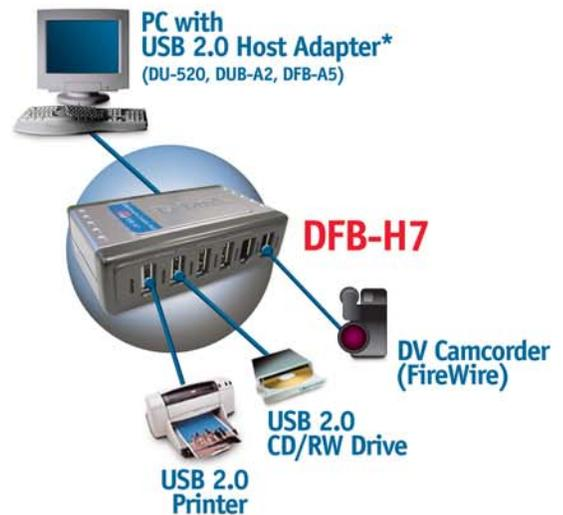
\*One FireWire Port and one Type B USB Port must BOTH be connected to a host computer or hub for all DFB-H7 ports to operate properly.
